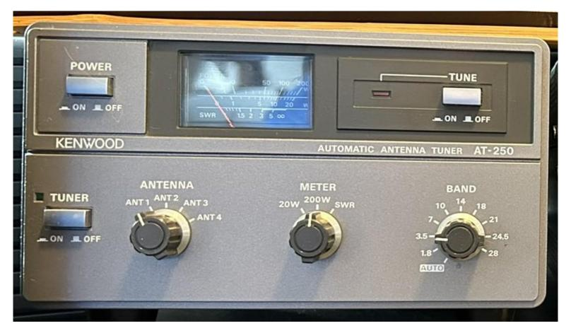
This unit makes a nice accessory for most any HF rig because it not only works on transmit AND receive, unlike the TS-450 internal tuner, and also covers the 160-meter band.
