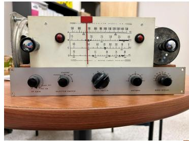
The unit needs a full recap, cleaning and alignment.
